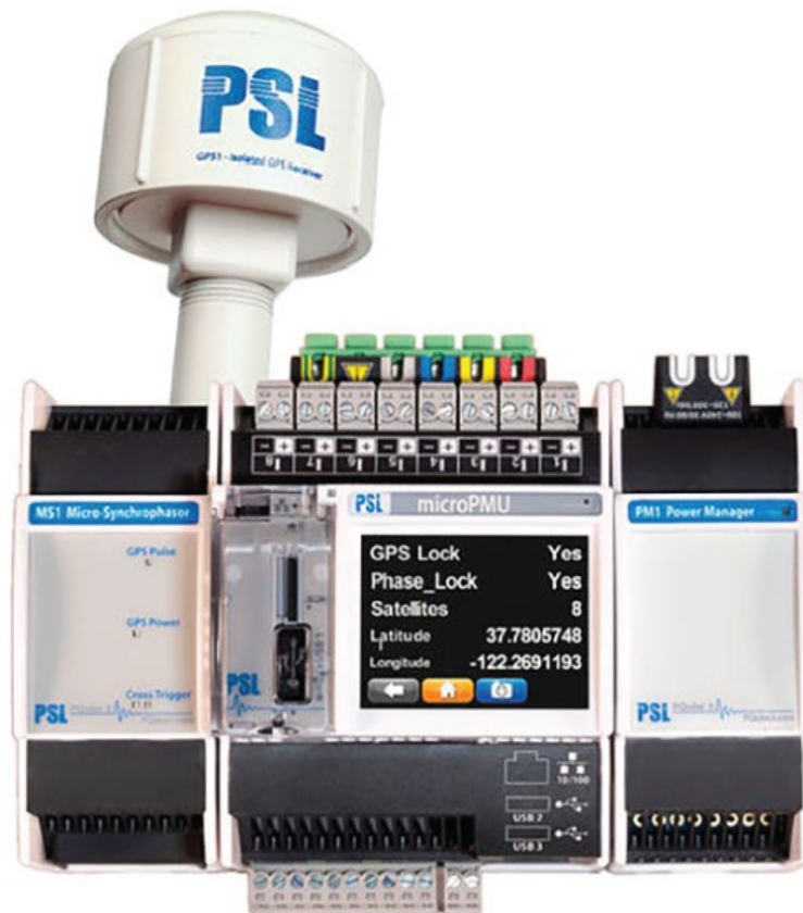
Fig: Micro-phasor measurement unit
